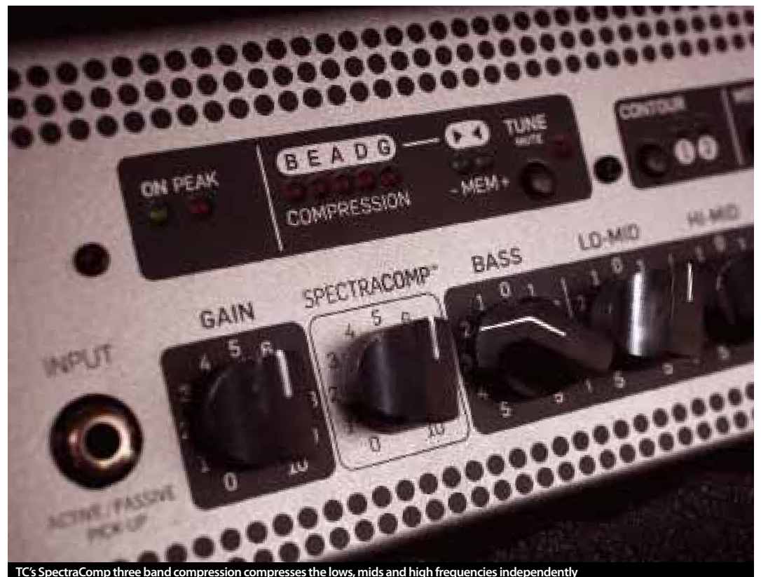
TC's SpectraComp three band compression compresses the lows, mids and high frequencies independently
