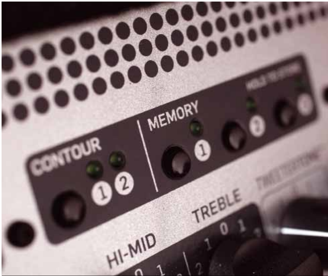
The three user memories can be saved and recalled at the push of a button
