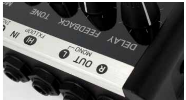
The Nova Repeater features stereo ins and outs to cater for two-amp setups
