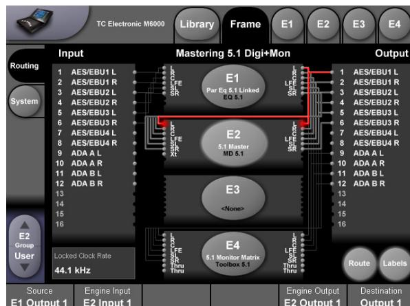
Fig. 5: Routing of inputs, outputs and processing blocks in the practical implementation [15].
