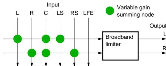
Fig. 3: Downmix matrix for 5.1 to stereo conversion.
