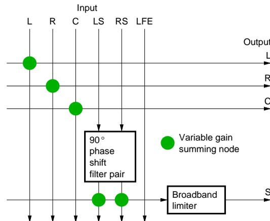
Fig. 4: Downmix matrix for 5.1 to LCRS conversion including a 90° mono filter pair.
