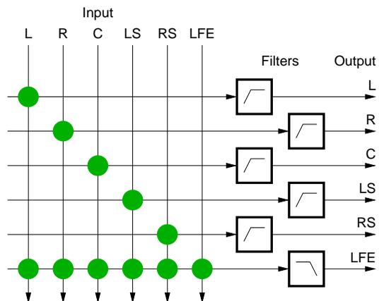
Fig. 2: Extraction of bass signal from the five main channels. The circles represent variable gain summing nodes.
