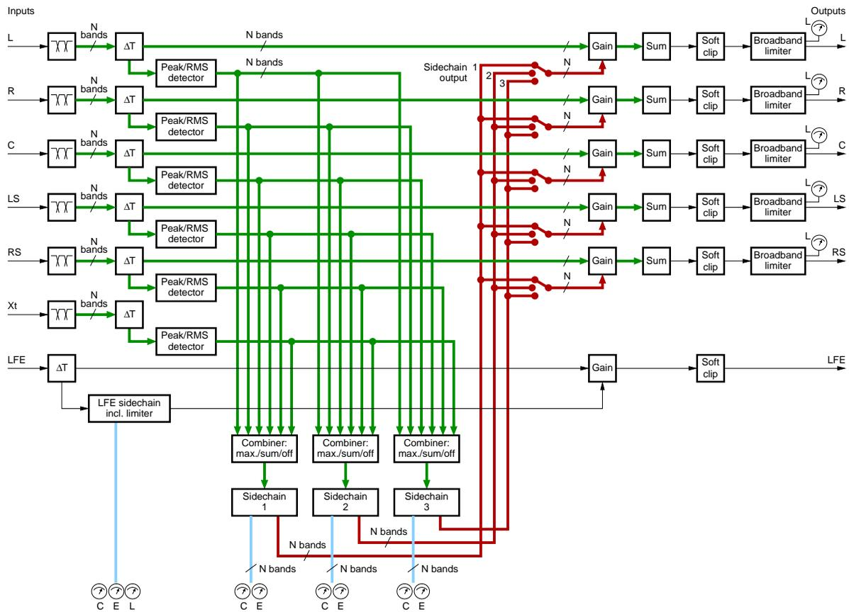
Fig. 1: Block diagram of a multichannel multiband dynamics processor. The number of bands,  $N$ , is 3.
